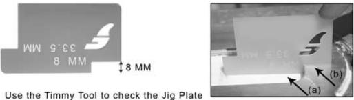
height. Flip the Timmy Tool over and place it inside of the jig plate so that the bottom of the Timmy Tool is flush with the blank (a) and the cut out part is flush with the jig plate (b). If it is not flush, use EVA shims underneath the jig plate to make adjustments. The plate height should be at 8 MM.
