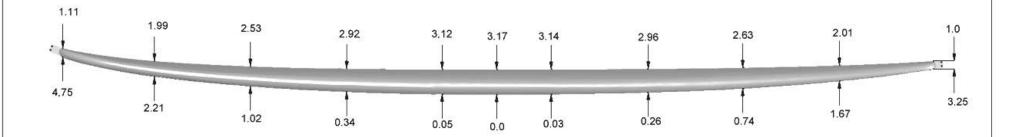
A very well balanced blank for hand shaping with room to move for cutting on the computer. Blank is shaped with a slight concave to maximize board design and thickness. NOTE:
