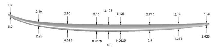
Blank is made to cut on computer.
