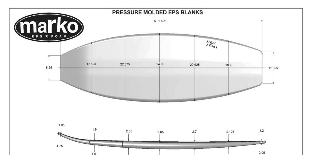
SHAPER'S COMMENTS: Fish Blank- This is close to 6' 2" C. Works great on machine. We are working to make this thicker
