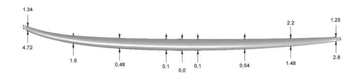
Blank is made to cut on computer. Blank has about 0.125 concave for maximum cutting ability. Ideal for Fishe and Hybrid shapes
