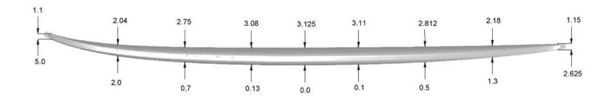
Ideal fun board blank. Can be cut, bent or altered to make other blanks for hand shaping or computer. Guns, short boards and/or fishes.
