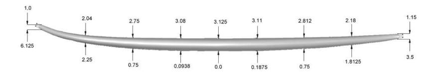
Room to move. Rocker bent to a magic 7' 4" gun. Ideal for both hand shaping or computer cuts. Bent to cut mid range boards 6' 8" to 7' 4" and room for the big guy board.
