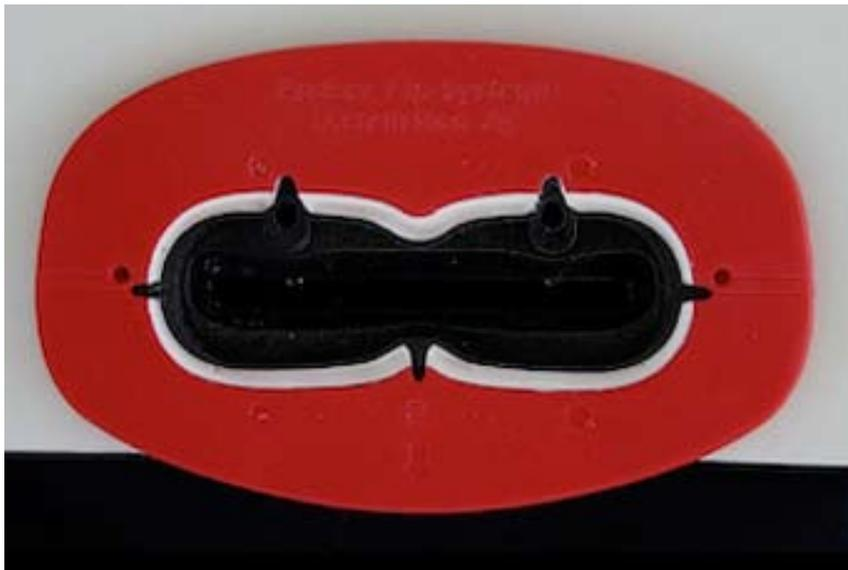
Add catalyst to the resin mixture and pour it into the hole until it is roughly 1/3 full of resin, now snap the box into the jig, it only fits one way. Push down on the **ProBox** to ensure that all of the tabs are down flush with the bottom of the board. It is critical that the **ProBox** be all the way down with all of the tabs touching the bottom of the board, this will ensure that the box is correctly aligned.
