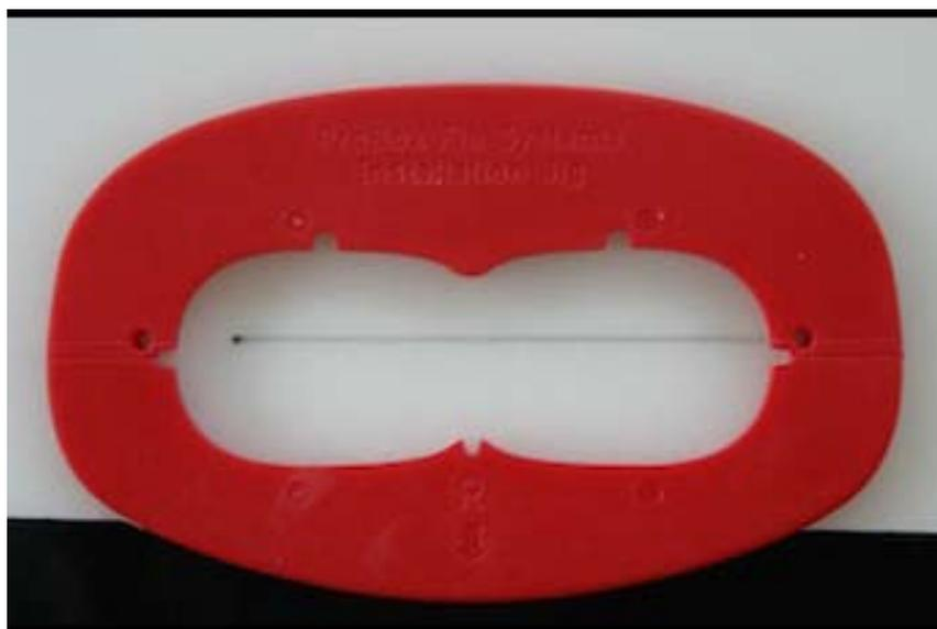
Prepare the installation jigs and the board by spraying a small amount of adhesive on the underside of the jigs and on the bottom of the board. A cutout masking template can be made from a piece of cardboard or door skin, using the jig as a template. This template can then be used to spray the adhesive on the board to minimize over spray.
