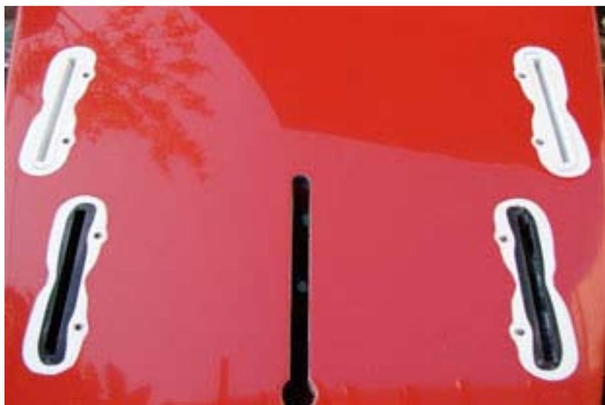
There are two preferred techniques for reinforcing the installation one of these techniques has to be used to reinforce the resin. These techniques are simple and effective and **do not** require milled fiber in the resin.
